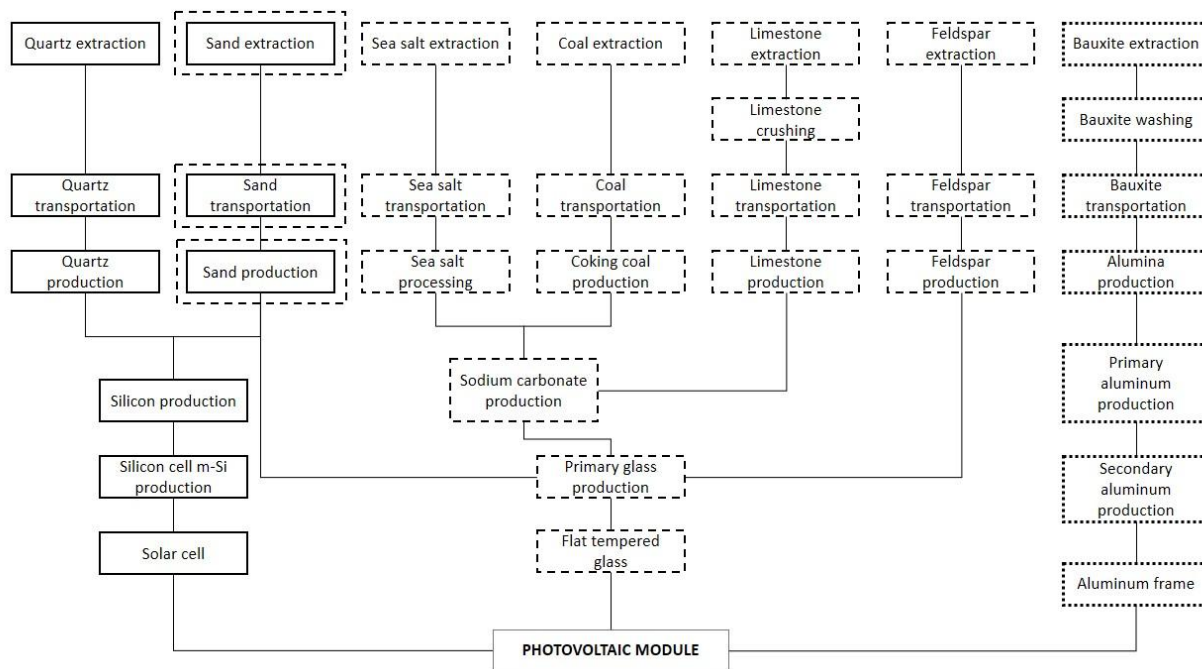
Fig. 2 - Flowchart of manufacturing processes of a m-Si photovoltaic module
